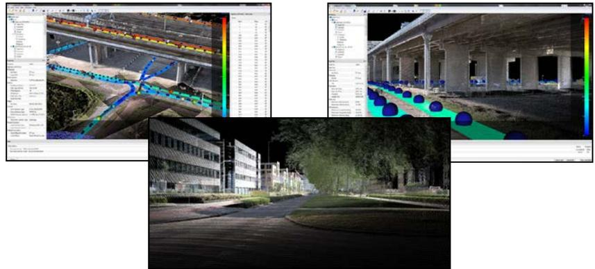
Mobile Master Office software provides a simple interface for combining, viewing, projecting and working with your various sensor data from the IP-S3 HD1 Mobile Mapping System.
