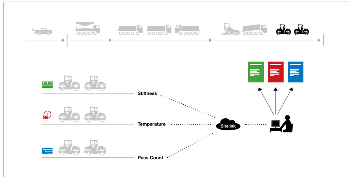
Fig. 13 - The Pavelink Compaction System
