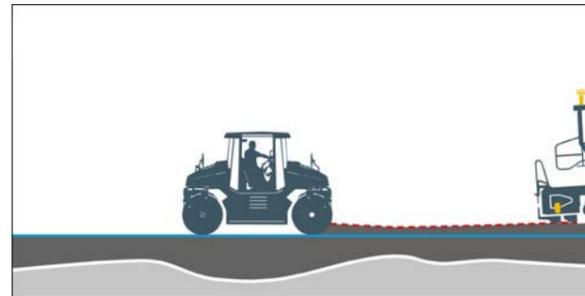
Fig. 6 - Compacting the Asphalt Layer
