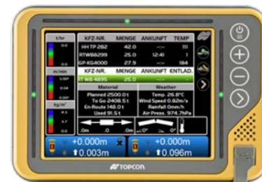
Fig. 7 - Operator View on the Paver with all Process-Relevant Information
