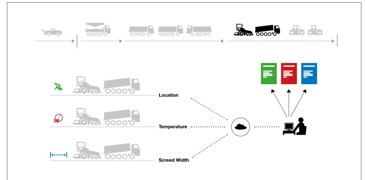
Fig. 12 - The Pavelink Paving System
