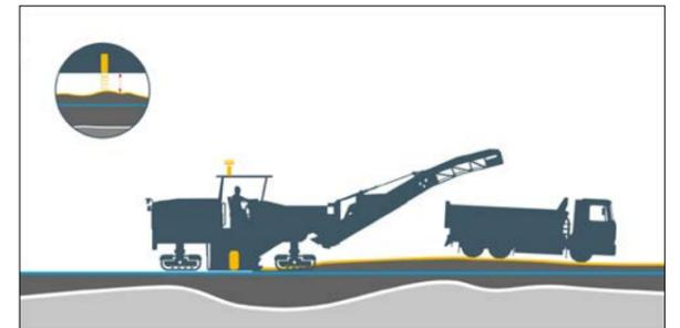
Fig. 4 - The Milling Process
