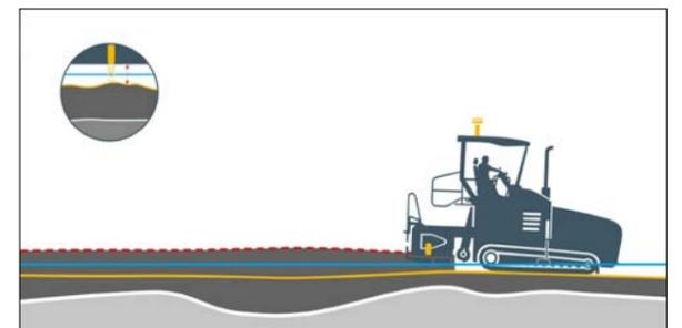
Fig. 5 - 3D Asphalt Paving
