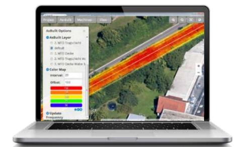
Fig. 10 - Recording of Temperature Measurements from the Rollers
