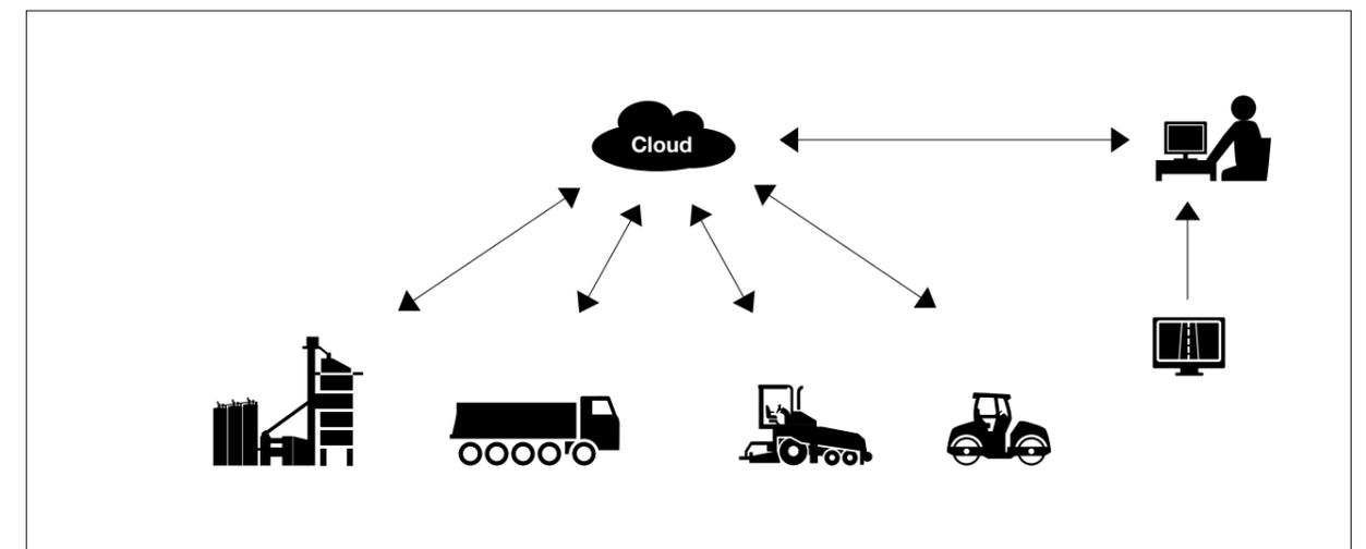
Fig.1 - End-to-end Model-based Control in Asphalt Road Construction
