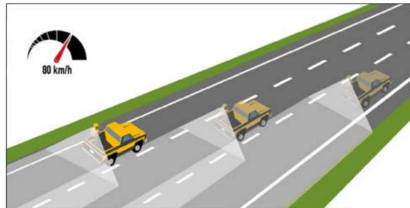
Fig. 2 - Mapping the Road Surface Using an RD-M1 Scanner
