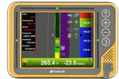
Fig. 9 - Operator View of the Roller Control Unit
