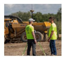
Like most survey personnel, once he steps on site, Arnold is barraged with requests which take him away from the work at hand. Meeting those requests used to impact productivity. That changed in 2019 with the addition of hybrid positioning, a software-based solution that allows his GT-500 total station to provide capabilities for both GNSS positioning and optical robotic measurement on one rover pole. With it, Arnold said, onsite distractions no longer became an issue.
