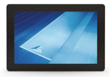
Compatible with many agricultural machines, the Topcon XC1 plus console provides a reliable interface in an economical yet durable form. This steering display features a 10" color touchscreen, high durability design for open-cab environments, and easy-to-use Topcon software with an optional ISOBUS unlock. Integrated with Topcon Manual Guidance and Value Line Steering solutions, the XC1 plus is ready for the variable needs of commercial agriculture.
