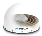
The CR-G5 is a choke ring antenna based on Topcon's TA-5 full spectrum GNSS antenna element. The TA-5 antenna element utilizes an array of vertical convex dipoles. This antenna provides Full Wave tracking technology for existing and future GNSS signals.
