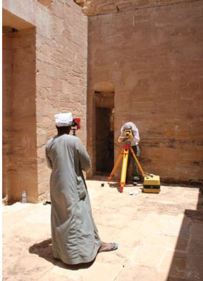
The Egyptologists use a digital imaging total station and advanced software to generate a virtual 3D model of the Ghueita Temple.
