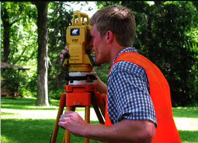
▲ A Purdue University student gets a backsight using a total station— courtesy Purdue University
